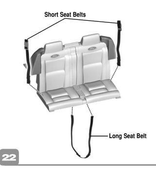
Insert the "T" fastener end of a short seat belt strap through the slot near the outer edge of the seat. Make sure the fastener side of the seat belt faces inward.
